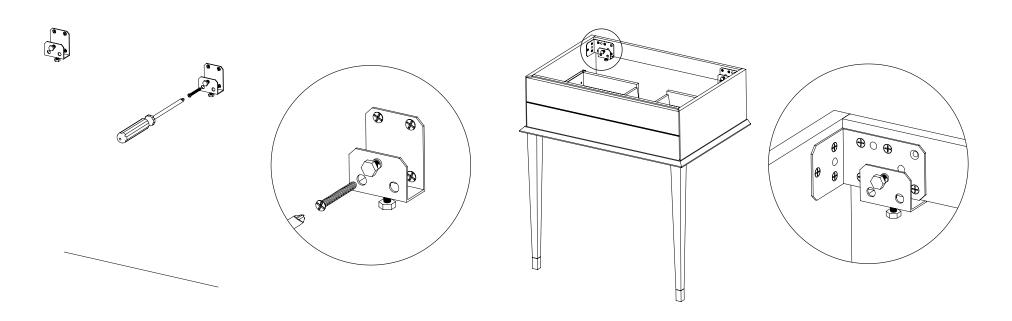
• Screw the Decofix system into the wall.
