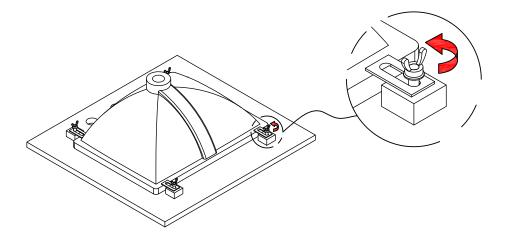
Place and tighten the screws in the aligned holes.
