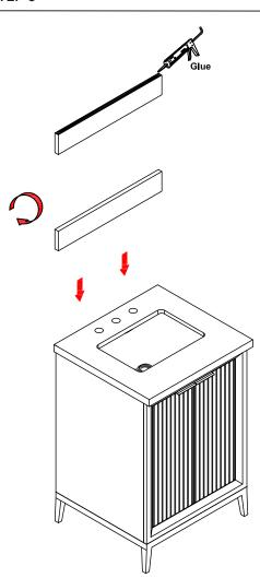
Apply caulk to the bottom of the backsplash and install so that the edge is flush with the back of the countertop.
