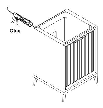
Apply caulk around the perimeter where the basin meets the countertop. Wait 24 hours for the caulk to dry fully.
