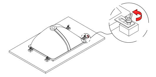
Place and tighten the screws in the aligned holes.
