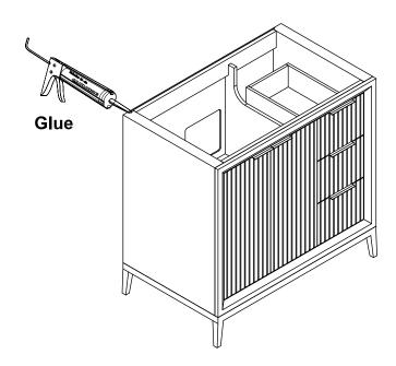
Apply caulk around the perimeter where the basin meets the countertop. Wait 24 hours for the caulk to dry fully.
