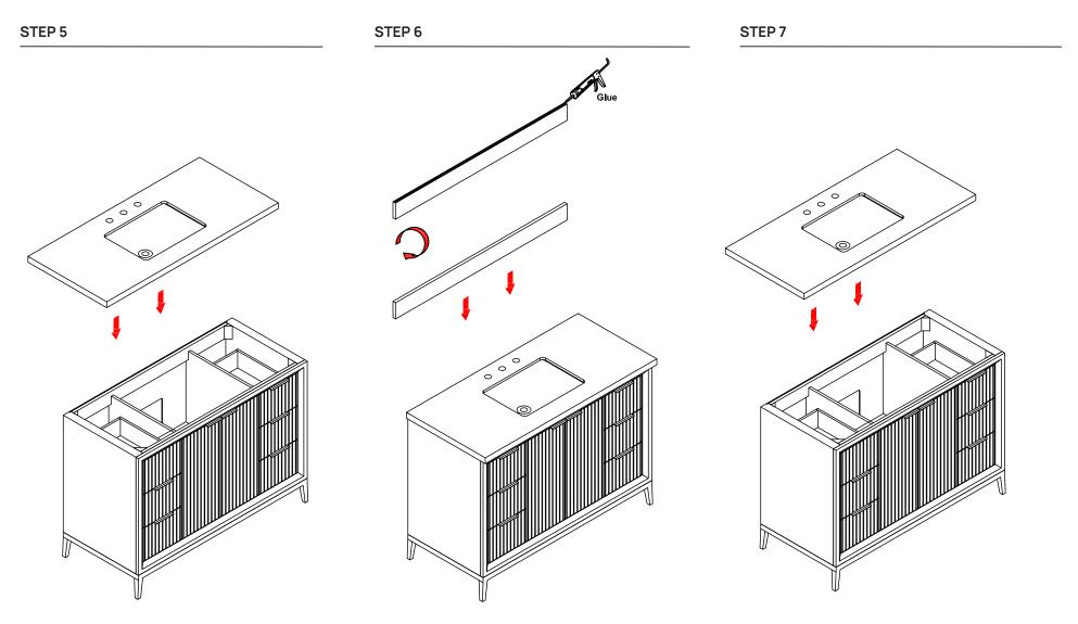
Install the countertop and attached basin so that the rim of the countertop rests on the caulk. Apply caulk to the bottom of the backsplash and install so that the edge is flush with the back of the countertop. Please allow the caulk to dry for at least 24 hours before using your vanity.
