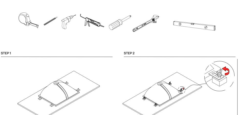
Set the countertop upside-down on a soft surface and place the basin upside-down on the countertop. Place and tighten the screws in the aligned holes.
