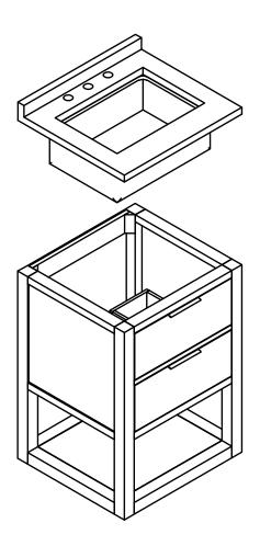
Install the countertop and attached basin so that the rim of the countertop rests on the caulk. \* Backsplash is included as a separate piece and is not attached to the counter. Installation is optional.
