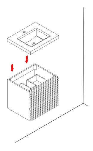
Install the countertop by attaching the basin so that the rim of the countertop rests on the caulk.
