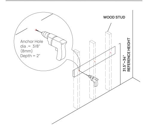
Locate the wood studs behind the walls. Mark the installation location for the wood cleat (C). Ensure the wood cleat (C) will be level before installing to the wall.
