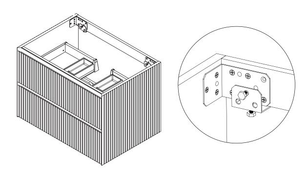
· Adjust the position screwing the screws.
