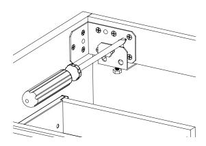
$\cdot$  Screw the main body to the wall in order to bring more security to the installation.
