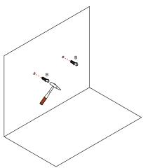
• White rubber plug for brick or concrete wall.
